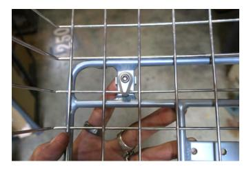
13. Finally, slide the tombstone-mounted block to the appropriate height needed to affix the chosen basket to the rack. Once you've done so, tighten down all three screws to secure both the tombstone mounting block and the two front mounting blocks.
