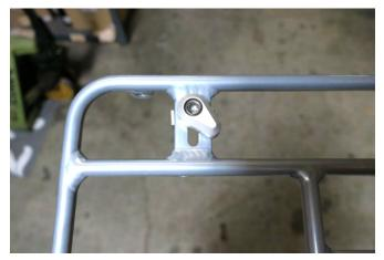
11. The large teardrop mounting block is attached using one (1) M5 x 16mm screw, one (1) washer, and one (1) M5 Nyloc nut. See photo for reference.
