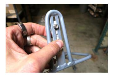
12. Leaving the front mounting assembly loose, center your basket on the rack, slipping a wire from the bed of the basket under the teardrop mounting block. The photo to the right has just one method of attachment. The orientation may vary based on the spacing of the basket that you're opting to use.
