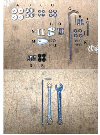
1. Snag two (2) sets of the 9mm spacers, eyebolts, M6 Nyloc nuts, & washers.
